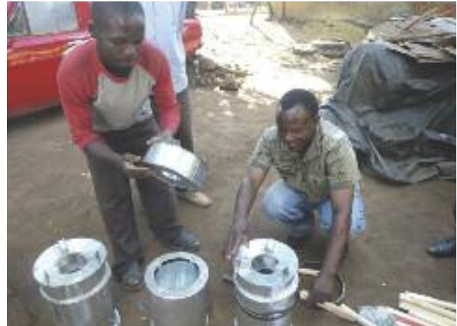
Figure 5. Local tinsmith Jonas (right) putting the finishing touches to the first prototype stove
