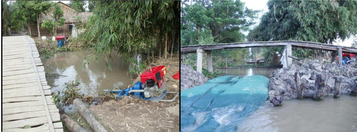
Picture 5-4. High-capacity pumps used in contracted pumping (pumps and pipes) (Subramanian 2011)
