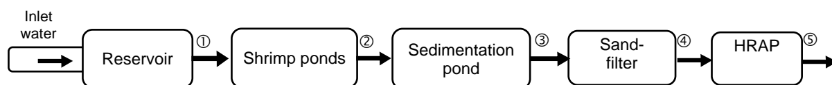
Figure 2. The water flow across the farm and the treatment steps used in the study
