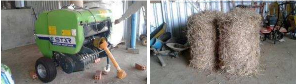
Figure 11: Straw baling machine available in the Mekong Delta (Galan, Japanese brand, Binh Chanh, province de Hồ Chi Minh)
